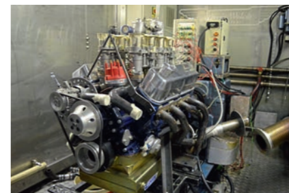
DWM has its own dyno to test engines after they've been rebuilt
